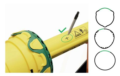
Please mark the selected position for later assembly with a suitable pen. For non-round guard tubes, select a position that is as flat as possible on the circumference of the guard tube (see illustration on the right).
