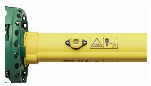
After you have checked the tight fit of the Counter, you can mount the shaft guard on the PTO shaft according to the manufacturer's instructions and then reinstall it on the machine. For the activation of the counter install the Walterscheid Connected Service App and follow the further instruction under "Add Counter".
