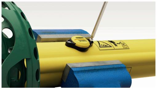
Carefully insert the screws into the Counter and tighten them with the Phillips screwdriver (tightening torque ~0.8 Nm).
