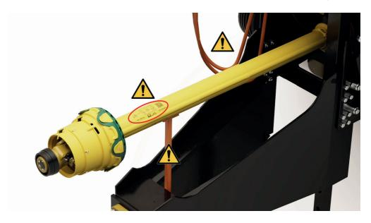
The selection of the appropriate position for the Counter is made on the machine with the PTO shaft installed. Select a position on the outer guard tube of the PTO shaft that meets the following criteria:
