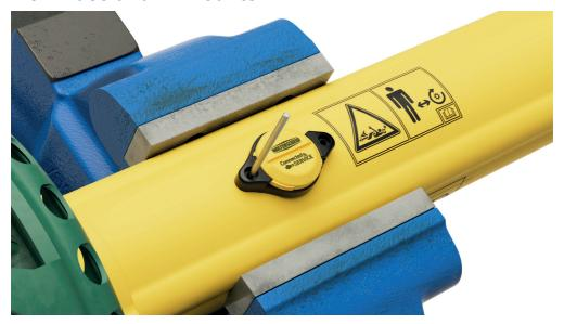
Fix the Counter at the previously marked position to use it as a drilling template. Then pre-drill the two holes with a Ø3 mm metal drill bit.
