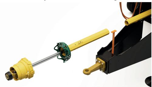
To prevent damage to the PTO shaft during installation, the outer part of the shaft guard must be removed from the PTO shaft. Disassemble the PTO shaft and the shaft guard according to the manufacturer's instructions.
