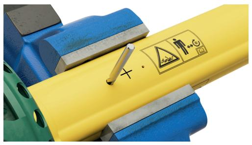
Remove the counter from the protective half and then drill out the two Ø3 mm holes with a Ø8 mm metal drill bit. Then remove chips and burrs.
