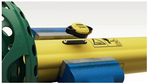
Carefully place the Counter on the mounting element. The metal hooks of the mounting element must be inserted into the bottom of the Counter housing.
